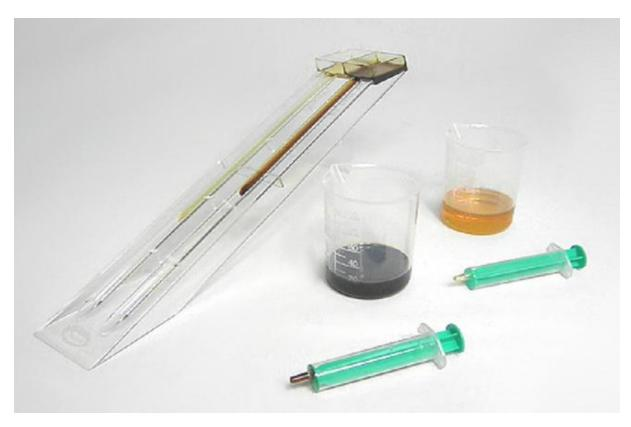
The easy-to-perform test procedure requires two oil samples of the same temperature (fresh oil and used oil) that are filled into different oil compartments. Once the fresh oil reaches the check point mark in a tilted position, the device is returned to the horizontal position. A quick "go/no go" answer of the test result distinguishes its principal application benefit as the viscosity of the used oil can be compared to the fresh oil sample and assessed immediately.
