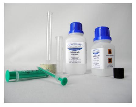
To determine the presence of acid in oil two reagents (indicator and titration solvent) are mixed until the green color appears. Then the oil sample is added, and the well-mixed liquid changes the color back to red if the acid is present.
