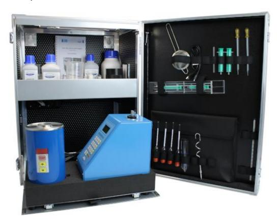
FUEL AND LUBE OIL TEST CABINET Basic Version incl. Reagents and Accessories
